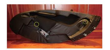
2) Take note each arm has multiple connections to be made. Air hoses need to be color matched. Electrical connections will be unique and only fit with their mate. Do not force.
